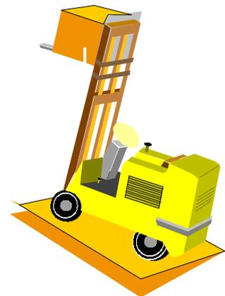
4. Travelling – with the mast at full rearward tilt and forks lowered, the forklift is tilted sideways on a platform to
