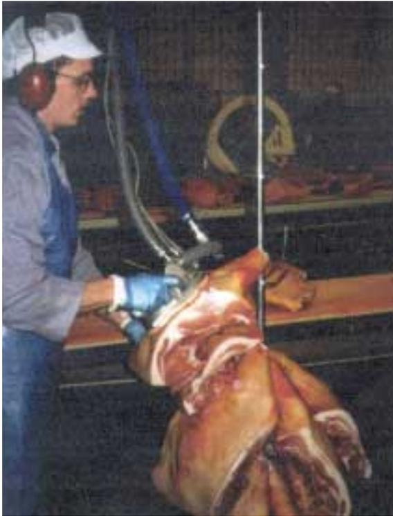
suction device and a pneumatic control unit. The operator places the suction device on the meat slab and a vacuum is created between the device and the item, so it can be lifted and held automatically for transport. By activating an open/close valve on the right hand side, the meat item may be raised and lowered without any heavy physical effort on the part of the operator.
