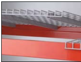
Left: wire deck; right frame spacers
