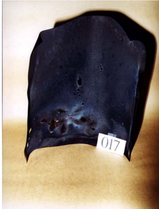
FIGURE 8. THIN-WALL CARGO LINER PENETRATION
