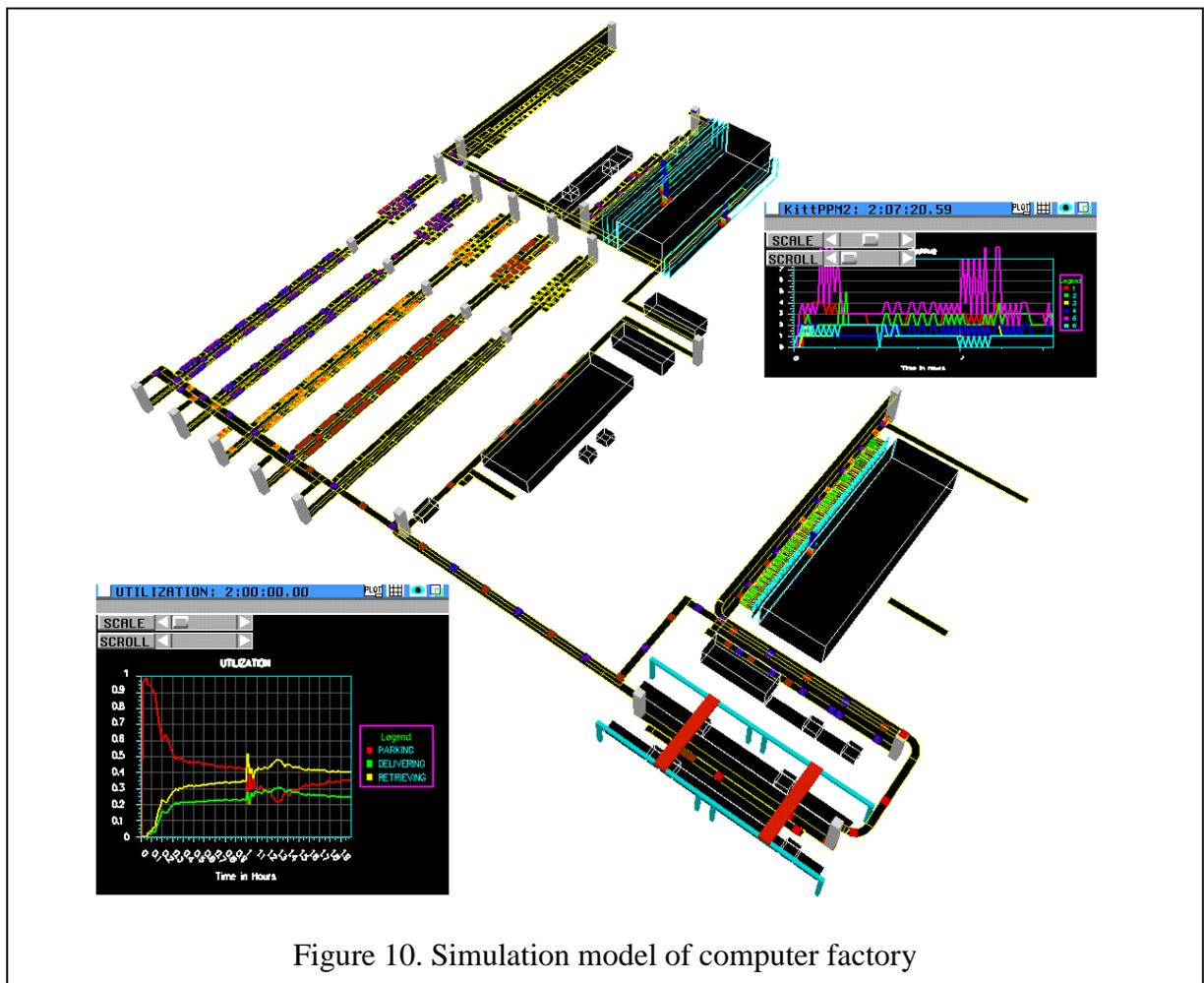
Figure 10. Simulation model of computer factory
