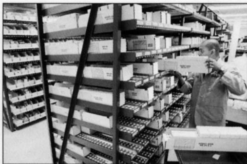
A Miltex employee re-stocks the gravity flow rack order-picking system which now guarantees first-in/first-out product flow.
